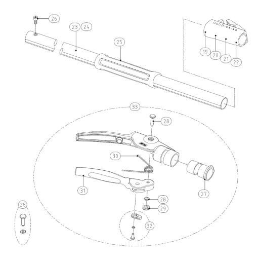
10. SP-ZF467 Joint case set for 160ZF203 31. SP-ZR349 Handle Lever Only 20. SP-ZF468 Joint case set for 160ZF305 32. SP-ZR380 Handle latch lock set SP-ZF469 Joint case set for 180ZF203 33. SP-ZR348 Handle Set (Includes everything 21. SP-ZF470 Joint case set for 180ZF305 22. inside of large circle above) 23. SP-ZF471 Lower Pipe Only, for ZF203 Lower Pipe Only, for ZF305 SP-ZF472 24. Middle Grip 25.
